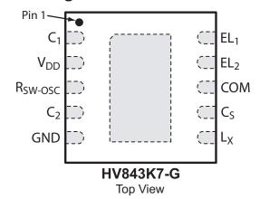
Note: Pads are on the bottom of the package. Back-side heat slug is at ground potential.
